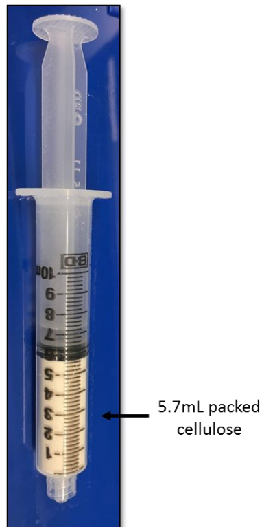
Figure 9 – Cellulose column used to deplete leukocytes and platelets from blood. 10mL syringes were packed with 5.7mL cellulose on the day prior to reticulocyte isolation.
