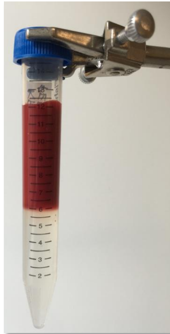
Figure 11 – Demonstration of layering blood over 70% Percoll cushion without any mixing or disruption of the interface (6mL mark on tube) between the two media.
